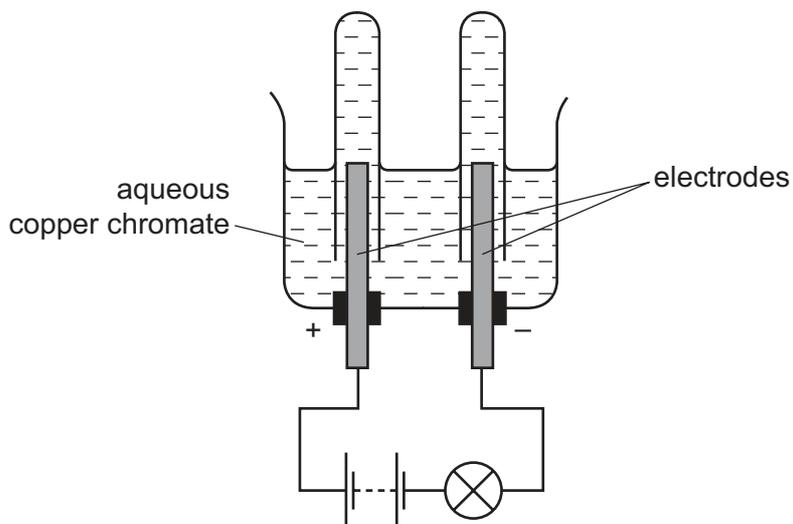
A brown deposit was seen forming at one electrode and oxygen was evolved at the other electrode.
